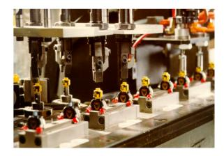
The clearest example of the assembly process is the minifig body or legs assembly. Each minifig body is made up of 5 parts that must be assembled: 1 torso, 2 arms and 2 hands. The process is very laborious in machine time terms as it requires several steps:
