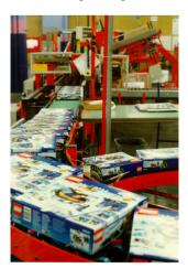
At the box packaging section, we start with completely disassembled boxes. The packaging machine folds the box, applies glue where necessary, puts the bags into the boxes, adds any large pieces, the instructions manual and decal sheet (if applicable) and finally closes it.
