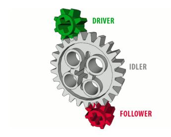
In the diagram above the large gray gear is meshed with the driver gear at one side and with the follower gear at the other. This is typical for idler gears: being meshed with many gears at the same time. Idler gears are usually meshed with two gears at the same time, while the driver and follower gear are only meshed with one. This is an easy way to identify idler gears, but there are exceptions.
