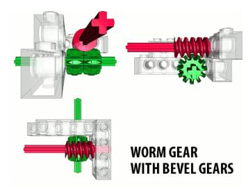
In the diagram above, two 12 teeth double bevel gears have been used. But it can be just a single double bevel gear, or two single bevel gears, or even just one single bevel gear. It's even possible to use the worm gear to drive racks, which may result in e.g. a very compact boom extending mechanism:
