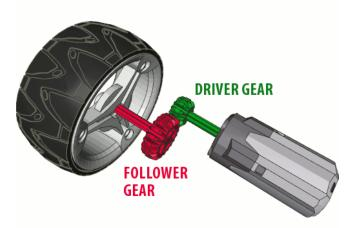
Almost every mechanism has its driver and follower gear. In every pair of meshed gears there is a driver gear and a follower gear. It should be sufficient to remember that the driver gear is the one the drive is transferred from, and the follower gear is the one the drive is transferred to.
