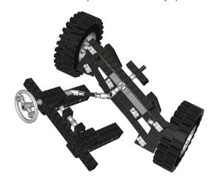
The rear axle incorporated a 3 speed gearbox. Since it was not synchronized it was difficult to fit the transmission shaft as it was almost never correctly aligned. One of the positions of the gearbox acted as a curious handbrake that immobilized the vehicle. I used to leave it on a tilted surface until the pitiful sound of the plastic of a TECHNIC gear or axle aroused my spirit of solidarity.
