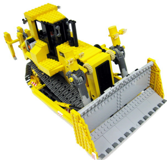
Caterpillar D9T model with just 6-studs wide hull. Some viewers are still surprised that it housed 5 motors, a regular battery box and two IR receivers. It had more functions than the legendary LEGO 8275 bulldozer, while being roughly 50% smaller.
