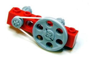
Belts are a simple and a relatively accurate alternative to gears if only small forces are involved.
