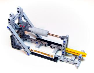
Linear actuators are a good choice where very precise movements are required. They can be additionally improved using some kind of a lever or a pantograph as shown here, where the yellow beam moves laterally with very high accuracy. Note the usage of friction pins in the mechanical parts too — they significantly reduce slack.
