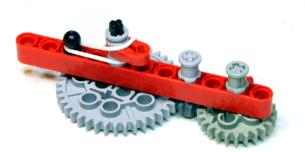
Backlash can be avoided by putting the entire system under a slight tension, usually at the last gear, as shown here on the 40-tooth gear with a rubber band.
