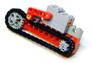
Chains are accurate and can transmit significant amount of force, but often need to be additionally tensioned, as shown in this example which uses a wind-up motor.
