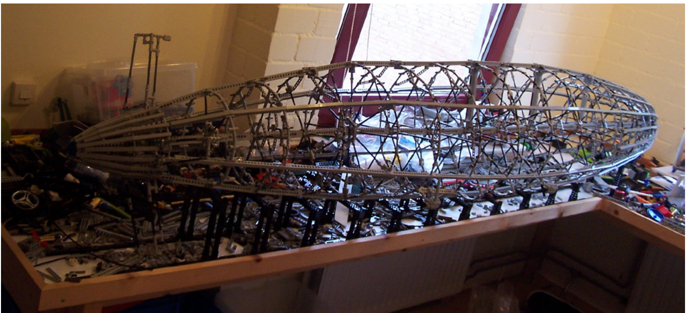
Figure 5: The outline is done, the model is resting with its belly on the black supporting structure. The stiffening triangles are visible at the edges of the rings (especially in front of the window).
