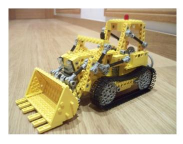
The elevation of the bucket as well as the mechanism for tipping it was controlled by two wheels at the back of the vehicle. The bucket was built with a couple of plates 4x12 and specific parts for the sides (Vehicle Tipper End) which appeared in black in set 912 and later in set 744. What sets are these? If the editors of this magazine keep on paying me as generously as they do now, I may talk about these sets at a later time.
