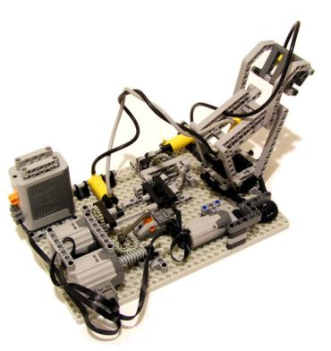
changes that appear on-the-fly. With this sort of baseplate, most of such problems are avoided as any component can be positioned literally anywhere — as long as it fits within the 31x21 studs constraints. Also, most Technic components, including motors and more complex parts, are easily and strongly connected to the baseplate using only a few friction pins — or axle pins if they happen to reside over an axle hole.
