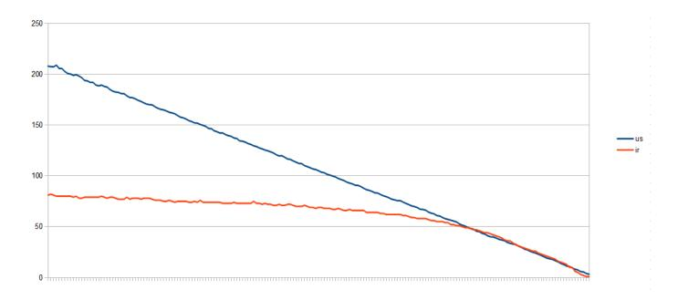
The first surprise when opening the files on the computer was that although the robot was at 2m from the obstacle when it started the initial readings never indicate anything over 85cm. This has been a constant in all the tests which has led me to believe that the floor affects the readings of the sensor. And it does: with the lower part of the infra-red sensor at 6 cm from the floor the distance it measures is always less than 85.
