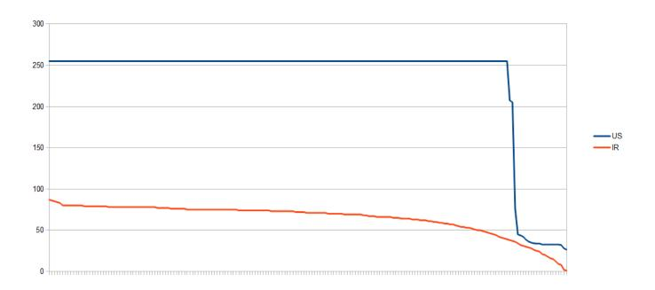
As you can see in this case the infra-red sensor is the clear winner sin the ultrasound sensor doesn't produce any reliable readings. I did another test using a box covered with a sweater and while the results were different the ultrasound sensor again did not offer any reliable results.
