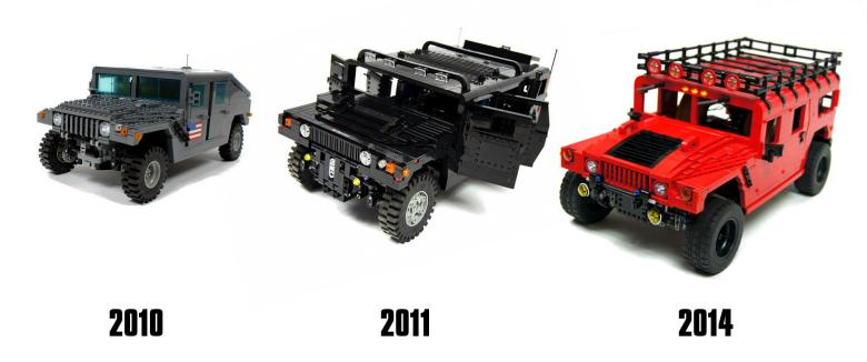
The model was built with two goals in mind: to look better than the two Hummers before it, and to drive better than my last large-scale off-road model, the Dakar Truck. Large scale enabled me to include some details that were missing from earlier models, while using PF system instead of the RC one made sure the model had plenty of torque needed for off-road driving.
