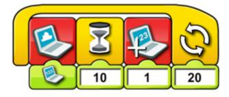
You will observe there is a Display Background block connected to the Display Input block. This means that the background displayed on the screen will correspond to the number shown.
