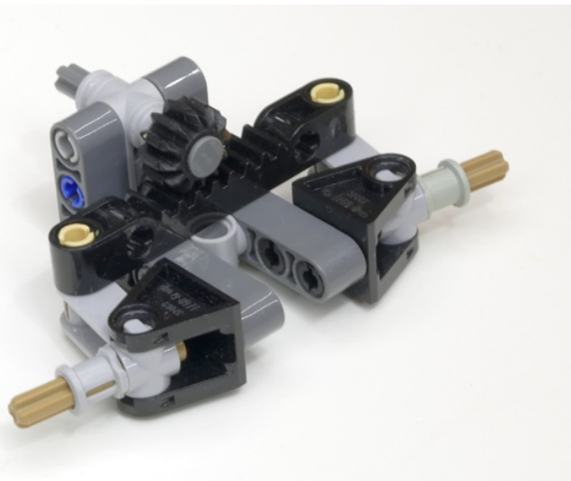
Using ready-made parts for simple steering allows for a very narrow chassis.
