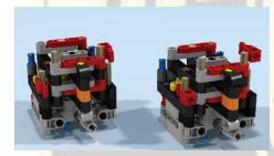
More important still is the fact that the slack in the gear changing mechanism can lead to two gears being engaged at the same time. EB user Attika realised this could be very easily remedied by placing the changeover caches in step 151 the other way round!
