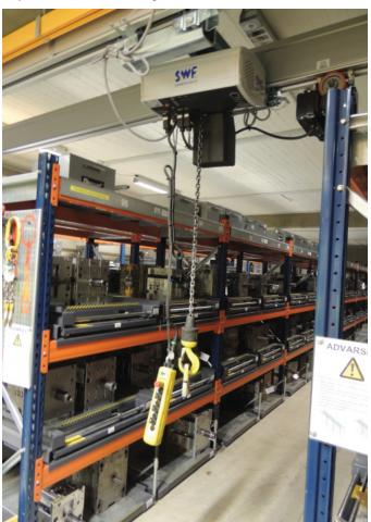
Finally we went to the chaotic warehouse, where the containers that come from the moulding machines are stored. A computer keeps track of where each part is stored and provides the necessary boxes when they are required. Each stand is 73 m long and 12.8 m tall. It is really impressive to see millions of bricks in the warehouse, and how the robots never stop storing and recovering containers. Oddly enough
