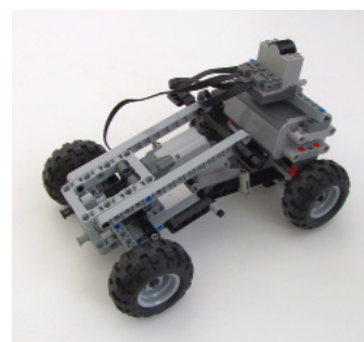
The rear drive and front steering configuration is the most common and can be built very simply and quickly, using just a couple of parts.
