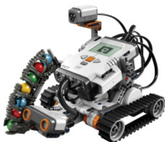
Differential drive, such as this official 8547 robot, allows turning in place, but steers roughly and with lots of skidding.
