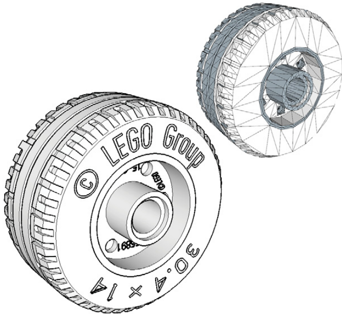
Fig. 4. Comparison between a part as imported (left) and the remodeled version (right) from my library. The level of detail I packed in includes tire text, part number and LEGO logo.
