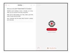
The first thing we will do is connect to the EV3 brick from within the Swift app. To do so, Tap the button, then tap "EV3 Brick". The iPad should connect to the EV3 brick and display EV3 Brick Connected.
