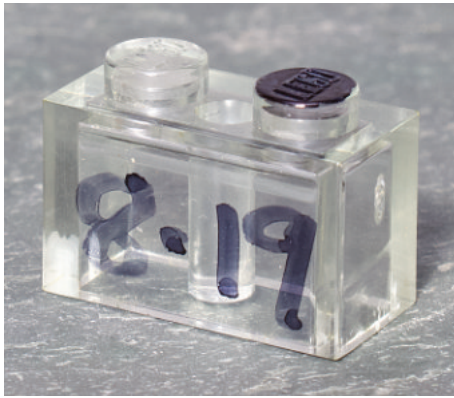
The 1x2 brick with underside bar prior to bleach bath. Writing on side is one-pass, ink on stud is multiple coats.
