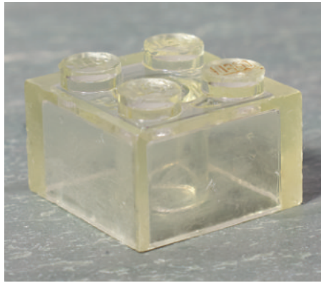
24 hours: Black on side completely gone, a little bit left around the edges of the logo on the stud. Plastic on sides has become noticeably cloudy.
