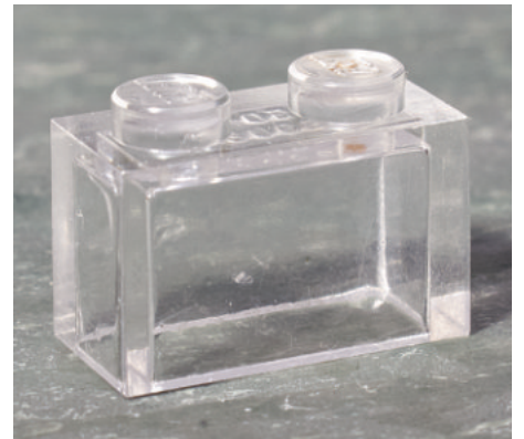
48 hours: Black on side completely gone, a little bit left around the edges of the logo on the stud. Plastic remains clear.
