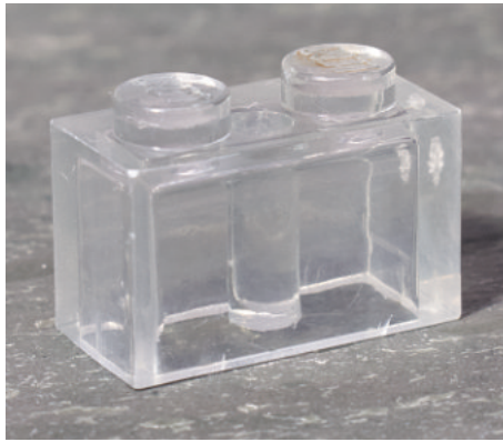
24 hours: Black on side completely gone, a little bit left around the edges of the logo on the stud. Plastic remains clear.
